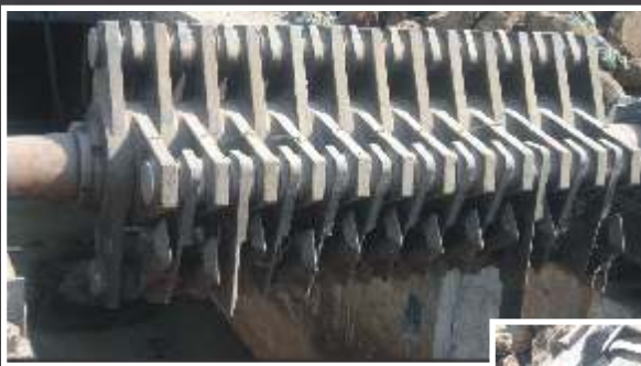
Complete Swing type Knife Assembly close view
